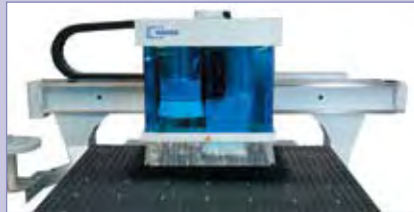
Strong 'gantry' design with internal struts for precision without vibration
